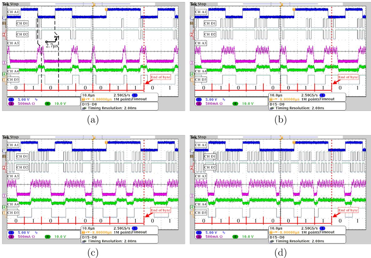
Legend: Analog channels: CH A1 (5 V/div) - DATA, CH A3 (500 mA/div) - Output Current, CH A4 (10 V/div) - Analog output of VLC receiver. Digital channels: CH D1 - PWM at switch  $S_1$ , CH D2 - PWM at switch  $S_2$ , CH D3 - Digital output at VLC receiver. Horizontal scale:  $10\ \mu\text{s}/\text{div}$ .
