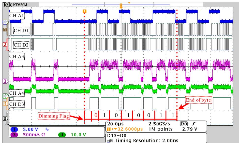
Legend: Analog channels: CH A1 (5 V/div) - DATA, CH A3 (500 mA/div) - Output Current, CH A4 (10 V/div) - Analog output of VLC receiver. Digital channels: CH D1 - PWM at switch  $S_1$ , CH D2 = PWM at switch  $S_2$ , CH D3 - Digital output at VLC receiver. Horizontal scale: 20  $\mu\text{s}/\text{div}$ .
