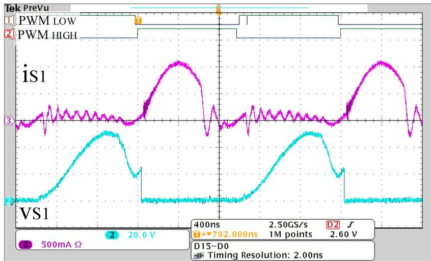
Legend: Analog channels: CH2 - Voltage  $v_{S_1}$ , CH3 - Current  $i_{S_1}$ .
