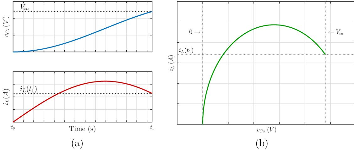
value. The remaining energy at the inductor is described through its current during the time  $t = t_1$ . The initial condition of this stage therefore is described by
