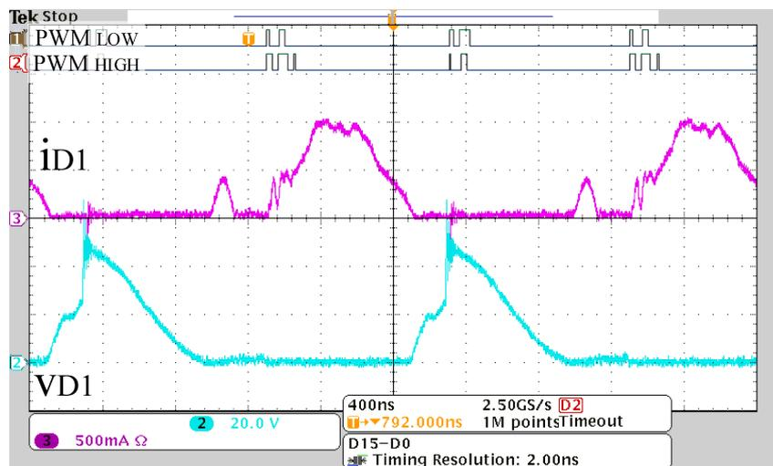
Legend: Analog channels: CH2 - Voltage  $v_{D1}$ , CH3 - Current  $i_{D1}$ .
