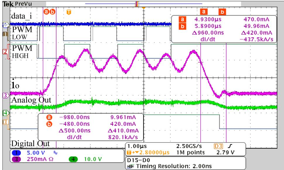
Legend: Analog channels: CH1 - Data transmitted, CH3 - Current  $i_{out}$ , CH4 - Receiver Analog Output. Digital channels: CHD1 - PWM LOW, CHD2 PWM HIGH, CHD3 - Receiver Digital Output.
