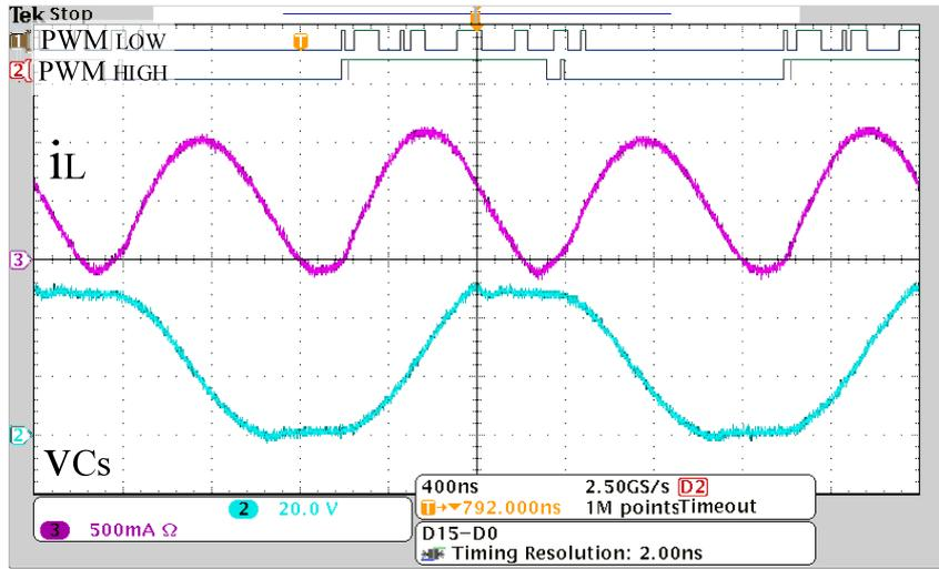
Legend: Analog channels: CH2 - Voltage  $v_{C_s}$ , CH3 - Current  $i_L$ .
