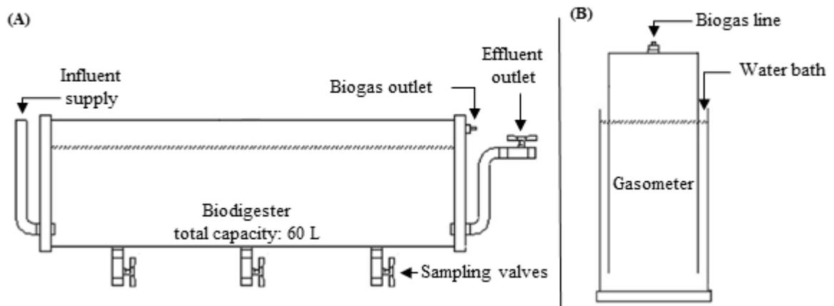
**Fig. 1 (A)** Anaerobic biodigester model; **(B)** Gasometer model.
