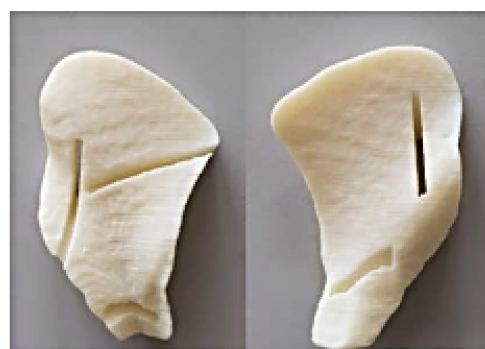
FIGURE 7: Final guide printed in ABS plastic (pelvic and abdominal faces).
