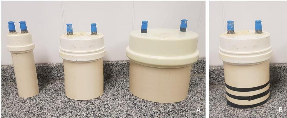
**Figure 1.** Polyvinyl chloride (PVC) opaque cylindrical chambers at sequence, from left to right: (A) Chambers with 5 cm, 10 cm, and 15 cm diameter. (B) PVC chambers depicting the three markings to assist insertion of the 10 cm chamber at depths of 1 cm, 3 cm, and 5 cm.
