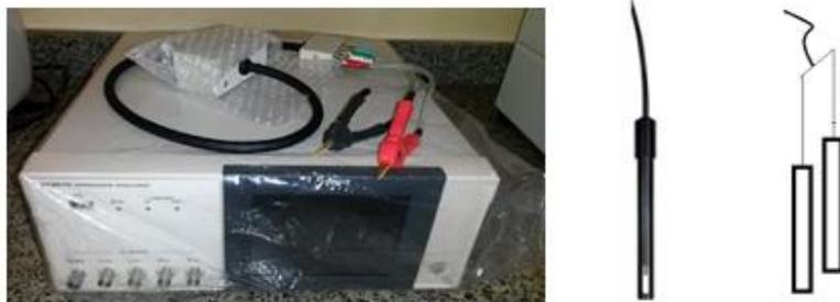
Figure 1: Simplified diagram of the geometry of a cell for measurements in liquids
