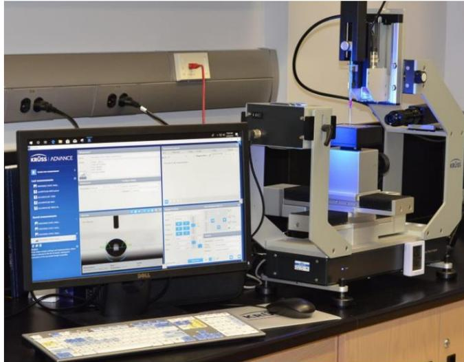
Figura 32 – Goniômetro (Drop Shape Analyser) acoplado ao software (Advance software)
