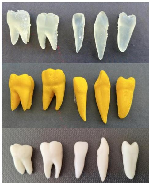
A-Teeth made by the Elegoo Saturn printer B: Teeth made by the Creality printer with yellow PLA filament (1.75mm), C: Teeth made by the Anycubic photon mono 2 printer.
