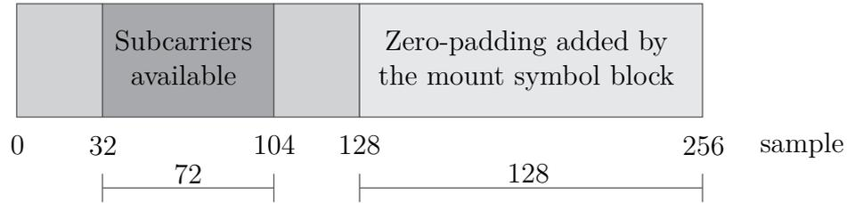
Figure 6: The OFDM symbol structure in frequency-domain.
