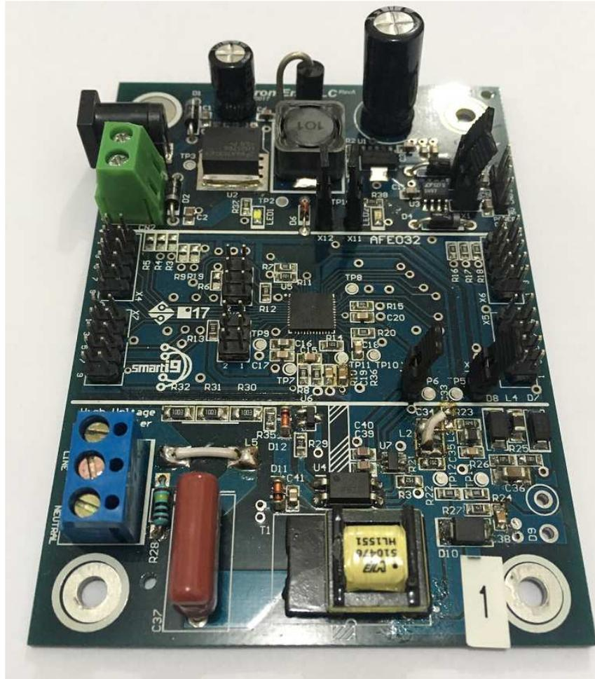
Figure 20: PLC analog front-end.
