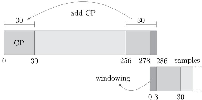
Figure 7: The OFDM symbol structure in time-domain.
