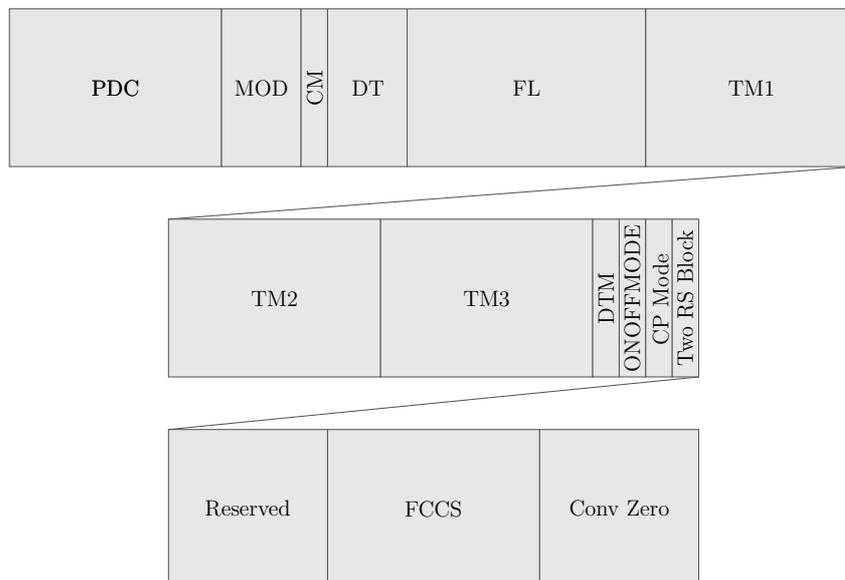
Figure 10: The structure of the FCH part.
