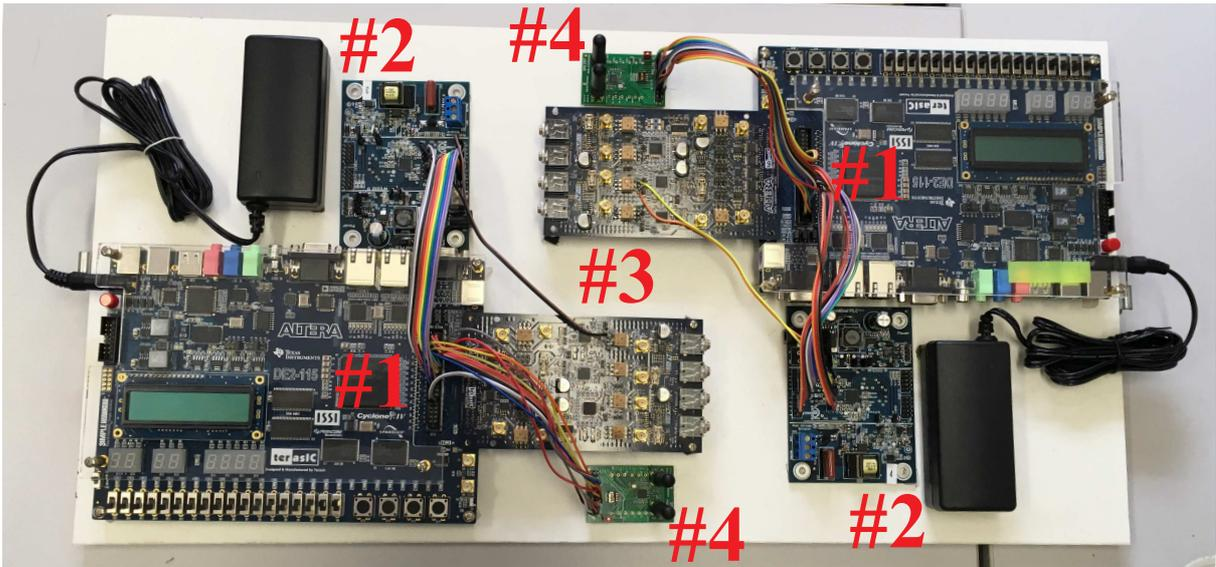
Figure 19: Setup of the NB hybrid PLC/Wireless transceiver prototype.
