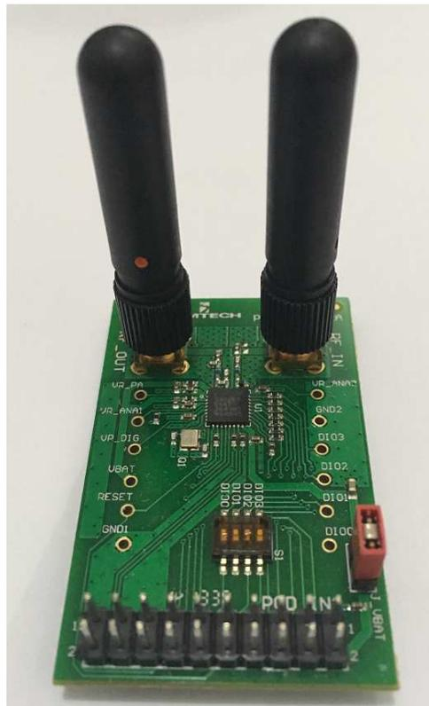
Figure 21: Wireless analog front-end.
