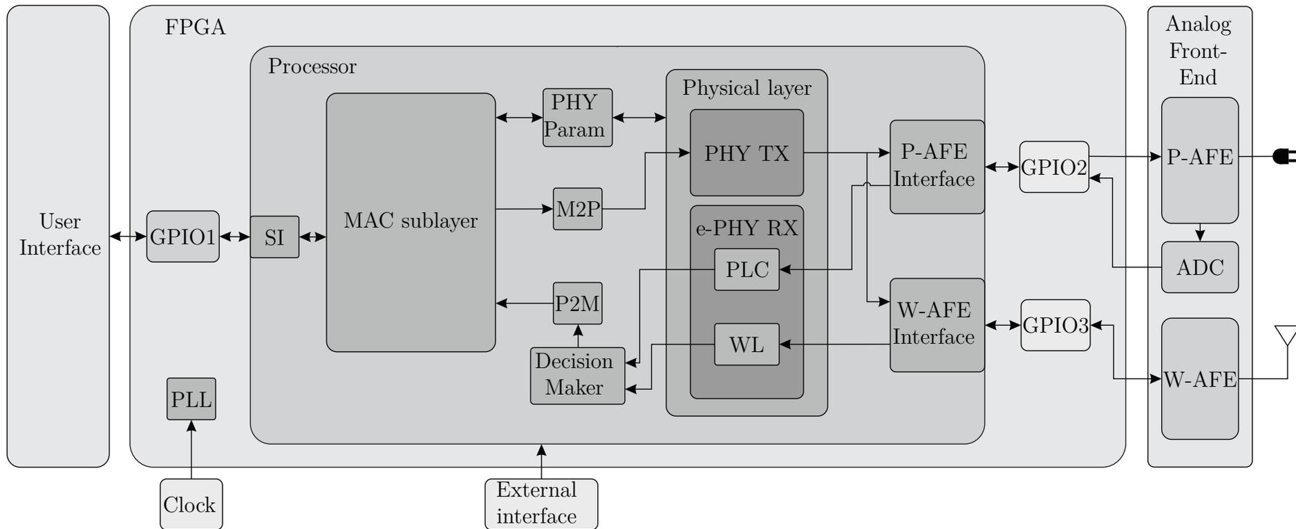
Figure 12: The block diagram of the proposed NB hybrid PLC/Wireless transceiver.
