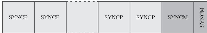
Figure 9: The structure of the preamble part.
