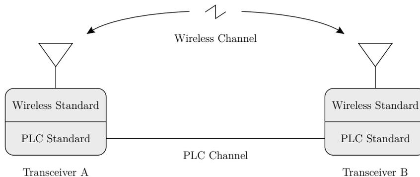
Figure 1: PLC and wireless approach.
