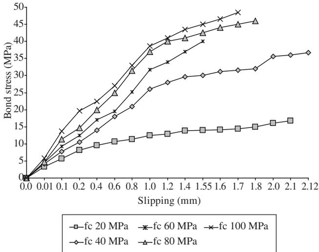
Figure 4. Bond Stress vs. Slipping ( $\phi = 20.0$  mm).
