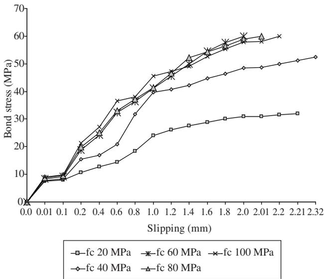
Figure 5. Bond Stress vs. Slipping ( $\phi = 25.0$  mm).
