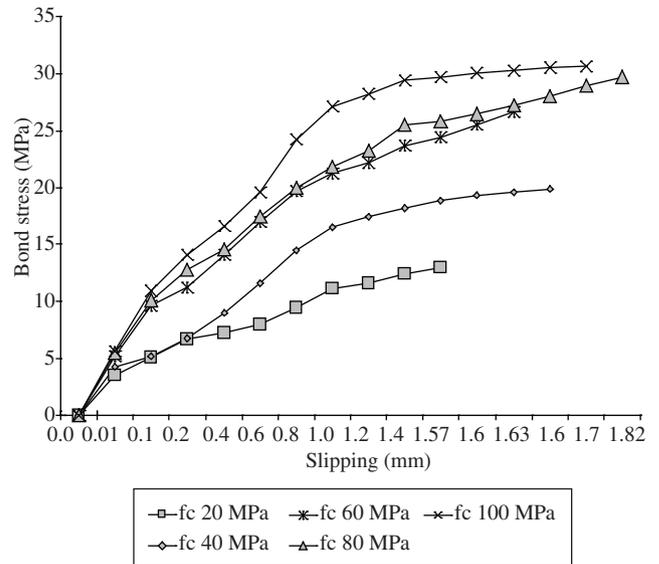
**Figure 3.** Bond Stress vs. Slipping (ϕ = 16.0 mm).
