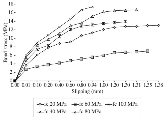
**Figure 2.** Bond Stress vs. Slipping (ϕ = 12.5 mm).
