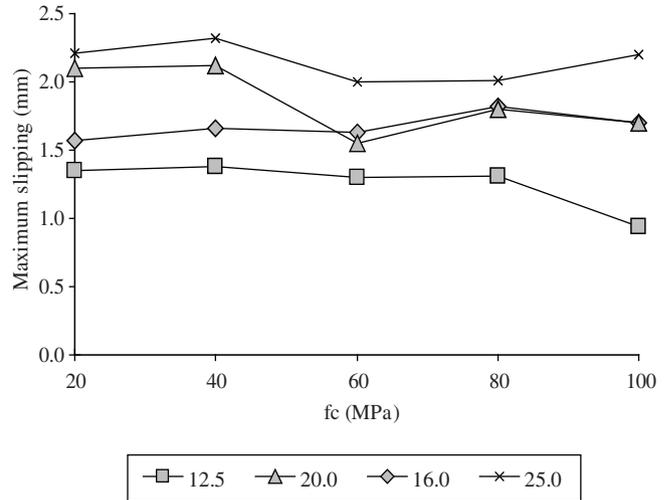
Figure 6. Maximum slipping vs. strength of concrete.
