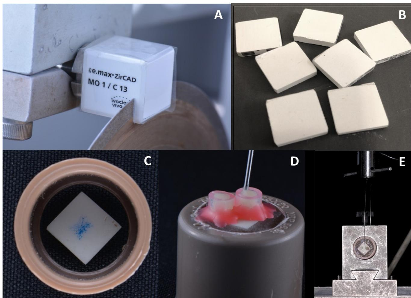
**Figure 1.** For the samples preparation, the pre-sintered YTZ-P zirconia blocks were sliced with a thickness of 2mm (A). These slices were polished and sintered (B). After the surface treatments, they were individually included in acrylic resin (C). After the resin cure, the cementation process started (D), for the subsequent execution of the shear bond test (E).
