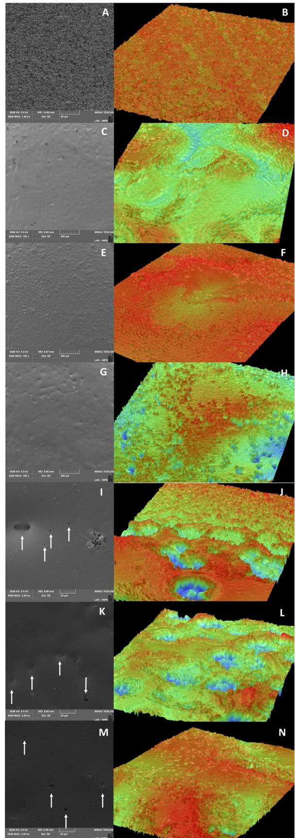
**Figure 3.** Micrographs (1000x) and 3D images of the surface roughness after the surface treatments. (A, B) Control group; (C, D) G5-5s; (E, F) G5-10s; (G, H) G5-20s; (I, J) G10-5s; (K, L) G10-10s; (M, N) G10-20s. The groups with the low-fusing porcelain glass layer etched with 10% HF have a rougher surface in the 3D images and the scanning microscopes show the creation of pores (pointed by the arrows) that can help in the micromechanical retention of the ceramic to the resin cement.
