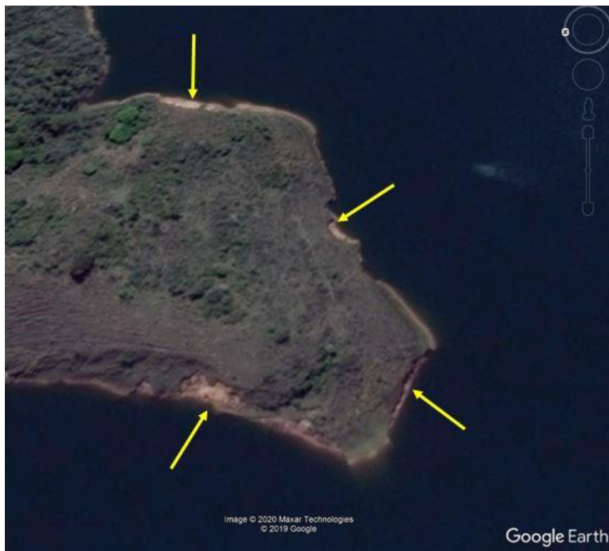
Figure 3: Example of erosion area by the margin of the CDU reservoir (Satellite image from Google Earth).
