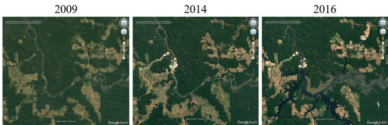
Figure 1: Modification of the ecosystem during and after the construction of the São Miguel Hydroelectric Plant on the Teles Pires River, located on the border of the states of Mato Grosso and Pará, Brazil. The figure shows three satellite images (Google Earth) before, during and after the construction of the dam. (2009): before damming. (2014): during the construction of the dam. (2016): after damming, showing the flooding of a vast region.
