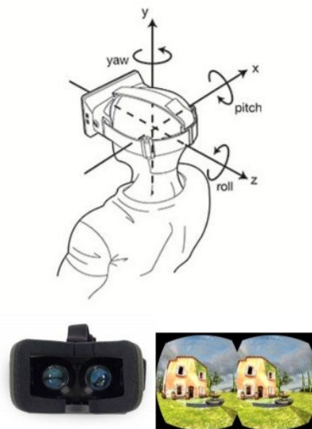
Figure 4 - Head tracking in the Oculus Rift Development Kit. Below, the illustration is the Oculus' headset (on the left) and the scene it is displaying (on the right)
