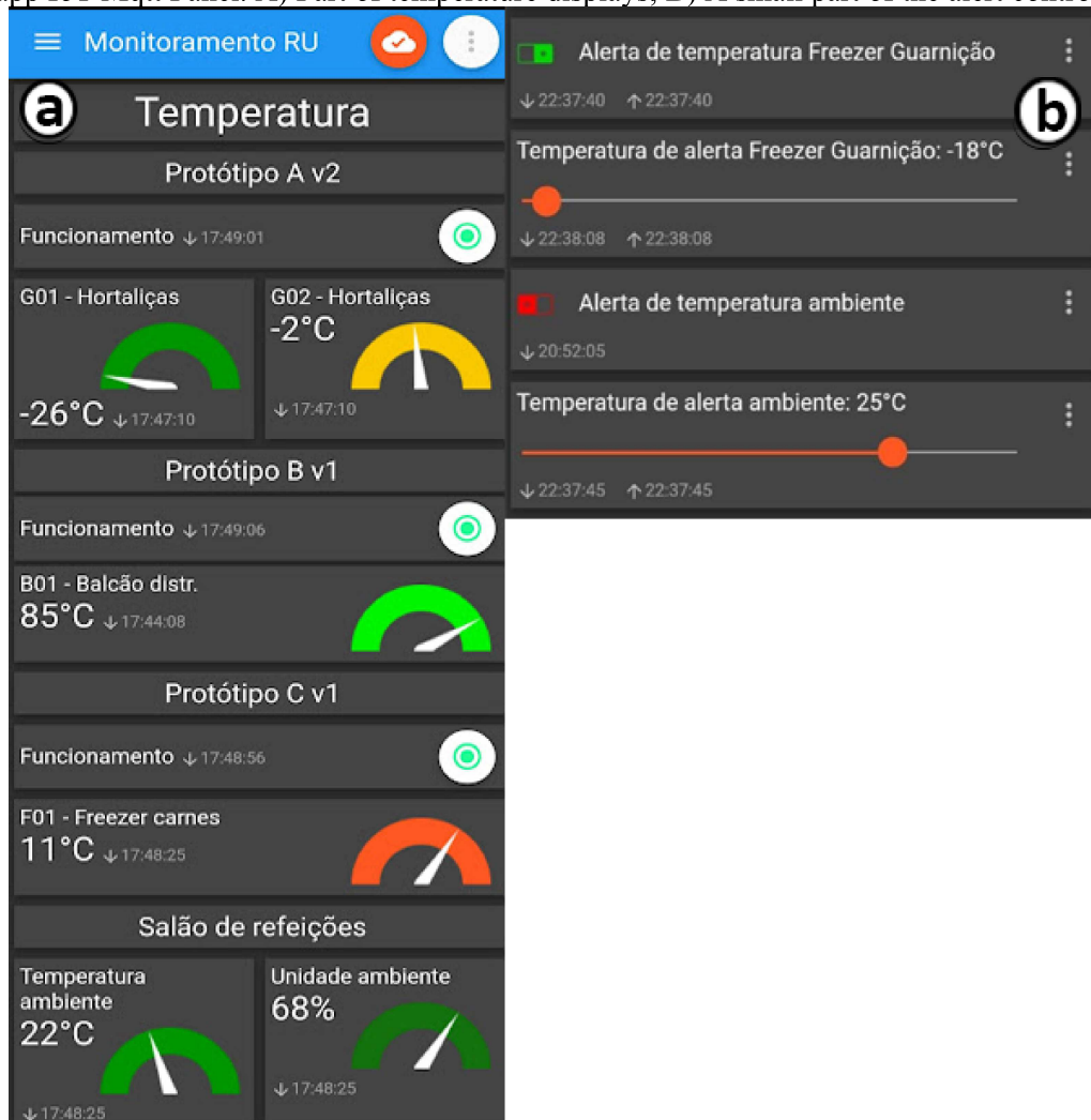
Figure 5 - Graphical interface in Brazilian Portuguese provided for FS managers through Android app IoT Mqtt Panel. A) Part of temperature displays; B) A small part of the alert controls
