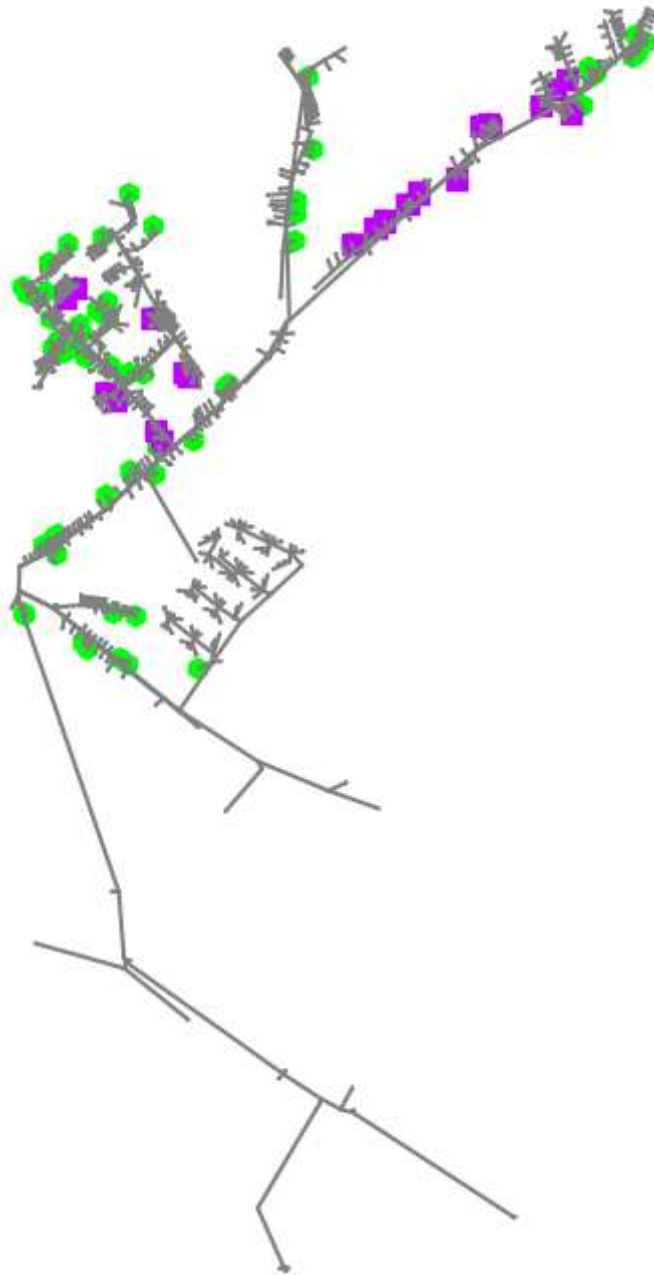
Figure 32 – Graphical representation of Case Study 02 energy community with batteries.
