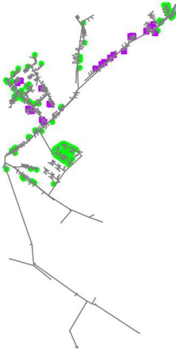
Figure 41 – Graphical representation of Case Study 04 energy communities with storage in the distribution network.
