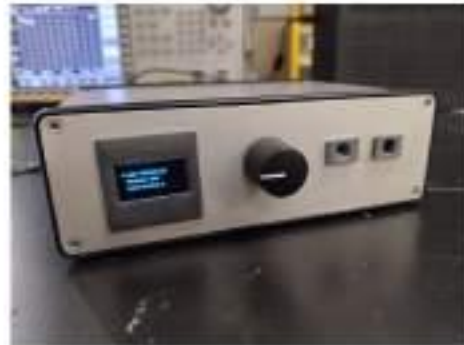
Figura 4. Low-cost light source developed at LITEL.
