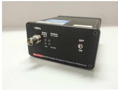
(a) E10-P portable rubidium frequency reference [44].
