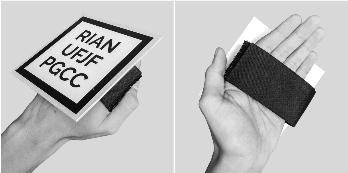
Figure 4.1: The first picture shows the AR marker on the back of the hand, which is used to display the virtual hand in the virtual environment, by the recognition of the marker pattern done via the smartphone camera and the VR system, thus providing a hand-based interaction within VR. The second picture is the same hand, but seen from the opposite side, showing the velcro.
