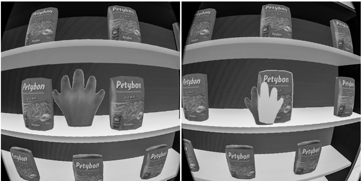
Figure 5.1: Virtual hand used for the hand-based manipulation in the case study 1. This figure shows a participant trying to select a product from the supermarket shelf using his hand through the augmented reality marker.
