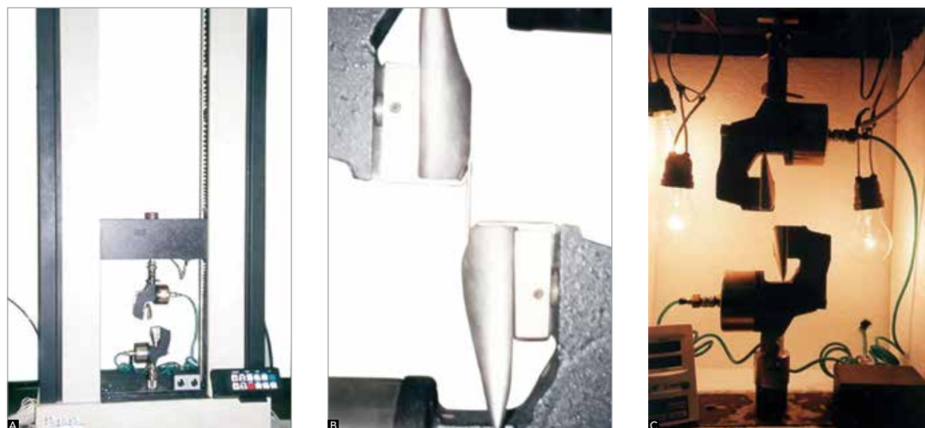
Figure 1 - A) Machine used on the performance of traction resistance tests, B) Detail of the wire tied by its ends to the machine's nails, C) Device used on the performance of tests at oral temperature ( 37^\circ\text{C} ).
