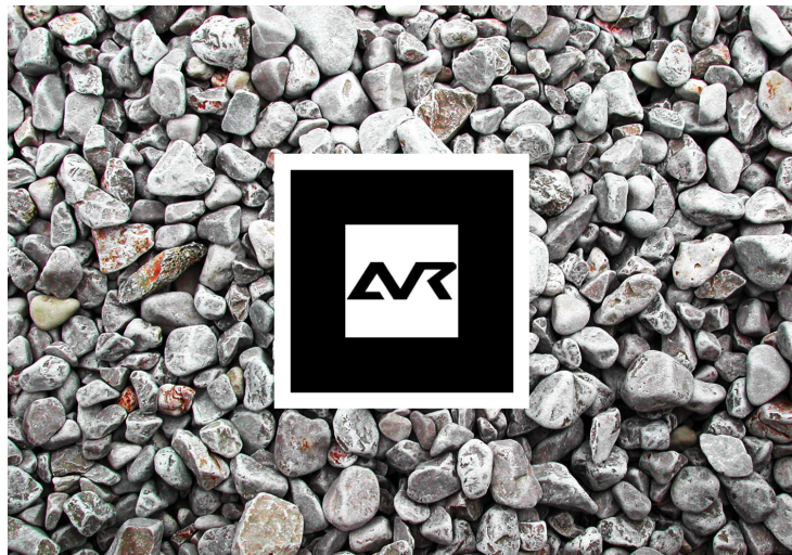
Figure 5.1: Marker object used in our sequences. The fiducial marker in the center has side s = 70mm , while the entire texture has dimension 24,7cm x 17,3cm.
